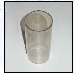
Production of diamond-coated guides. The photo on the left shows a laser beam evaporating a graphite target. The laser is so powerful that the evaporated graphite forms diamond bonds on the inner surface of the quartz guide (right image). This process produces guides with highly uniform surfaces—a feature critical for UCN transport.
